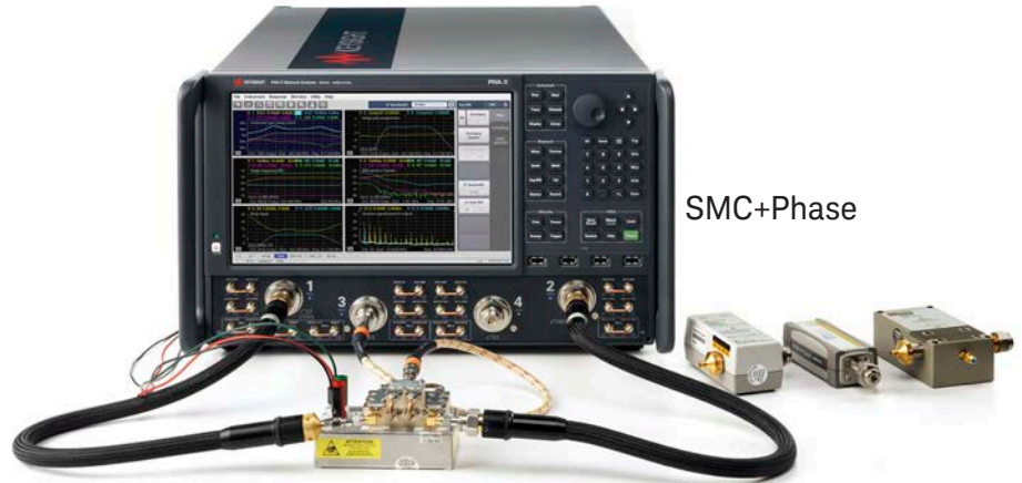
S93083A Scalar Mixer/Converter plus Phase (SMC+Phase) makes mixer and converter measurements simple to set up since reference and calibration mixers are not required. Calibration is easy to perform using three broadband standards: a power meter as a magnitude standard, a comb generator as a phase standard, and an S-parameter calibration kit (mechanical or ECal module).
